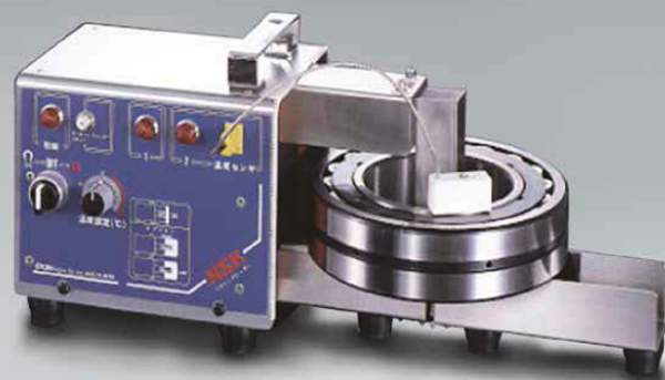
Fig. 5: Heating by bearing heater
