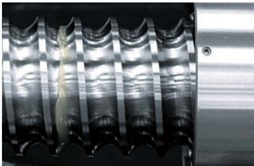
With grease retaining A1 seals
